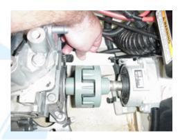
Reconnect the positive starter wire, and the start/stop wiring harnesses.
