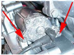
5.7 (Above) Use a 10mm socket to remove the two bolts securing the starter to the case, and pull it straight back.
