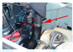
3.4 (Below) Remove the water line from the pipe and the head.
