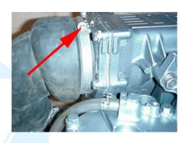
3.6 (Below) Remove the three 12mm exhaust muffler mounting bolts from the bracket and remove the pipe.
