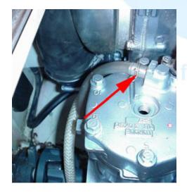
3.3 (Below) Remove the exhaust hose from the pipe using a screwdriver.
