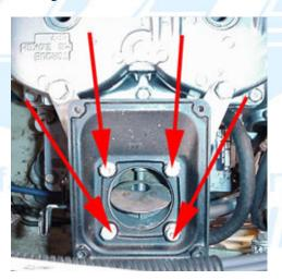
2.3 (Below) Loosen the gas tank cap to relieve pressure. Be sure the fuel switch is turned to the "OFF" position, and be aware of any fuel that may spill from the hoses. Make sure the hull is clear of any gasoline fumes before continuing work, especially with power tools. Remove the pulse, fuel in and fuel return lines from the carb.
