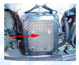
2.2 (Below) Remove the four 10mm bolts securing the flame arrestor base to the carb.
