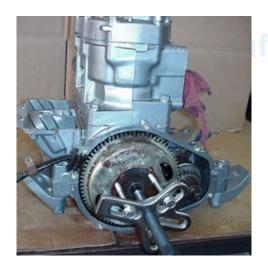
5.5 (Below) Use a screw driver to remove the two screws securing the stator assembly to the case.
