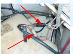
Disconnect the positive wire at the starter with a 10mm socket.
