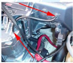
3.5 (Below) Loosen the clamp on the pipe to manifold coupler and remove it from the pipe. Fold back the outer flap for easy access.
