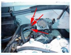
Disconnect the choke and throttle cables from the carb. Remove the two 10mm nuts securing the carb to the manifold and remove it.
