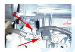
3.2 (Below) Remove the head cooling inlet line.
