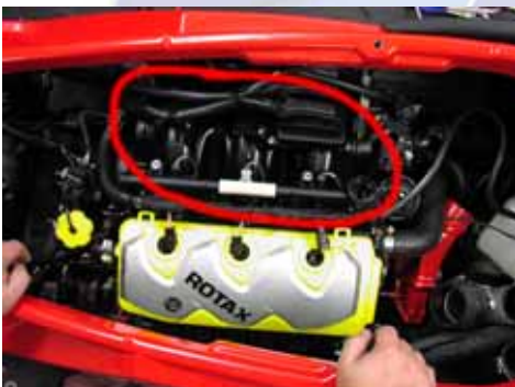
2.10 Remove the intake manifold. All the screws are hidden.
