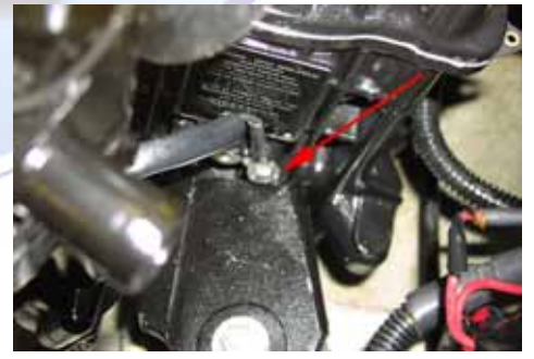
2.13 Remove the motor mounts the 3 rd mount is hidden.
