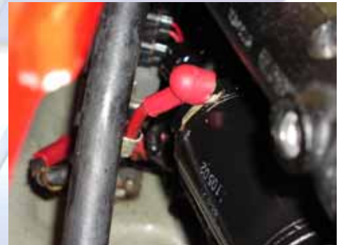
2.14 Hoist the engine with a cherry picker 6" for access. Remove the grounds and starter cables.
