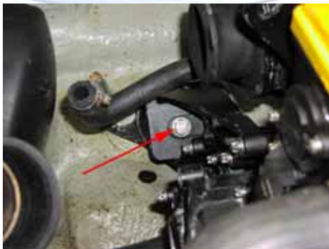
2.13 Remove the motor mounts the 3 rd mount is hidden.
