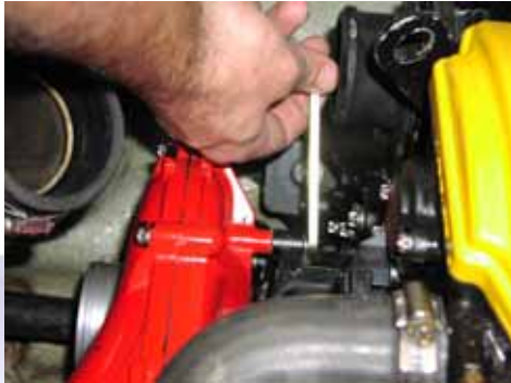
2.11 Remove the supercharger using the special wrench. The two bottom bolts are hidden.
