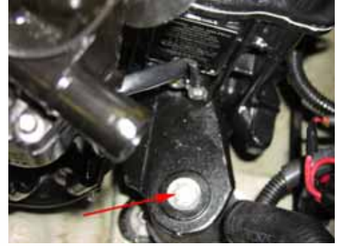
2.11 Remove the supercharger using the special wrench. The two bottom bolts are hidden.
