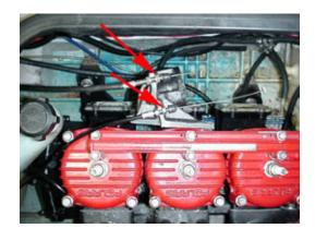
3.11 (Left) Inspect each reed assembly for damage and wear. Look at each reed petal and inspect the edges for signs of cracking, chipping or any missing parts. If any damage is present, replace the petals.
