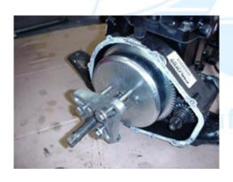
6.5 (Above) Remove the end nut on the shaft with a 19mm socket. The rag in the exhaust port for PTO coupler removal will again prevent the engine from turning over, allowing the nut to be removed. Next use a universal flywheel puller to remove the flywheel from the shaft. **CAUTION:** Do not screw the puller screws into the flywheel more than 5 complete turns or damage to the stator may occur.
