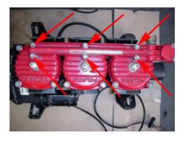
6.3 (Right, Below) Remove the two bolts securing the oil pump to the flywheel cover with a 8mm socket. It is SBT's recommendation that the oil pump be left off the new engine, and a block-off plate be installed at this time. Remove the seven flywheel cover bolts with a 10mm socket.
