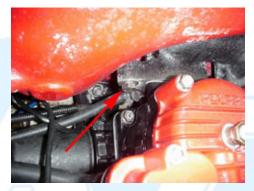
4.3 (Left) There are 2 lower bolts securing the exhaust pipe to the exhaust manifold. Remove the rear bolt using a 17mm socket.
