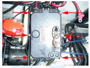
5.3 (Above) Open the electrical box by removing the six bolts with an Allen wrench.
