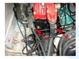
4.7 (Below) Remove the temperature sensor by removing the retaining nut with a 8mm socket. This will allow the mount plate to be removed, exposing the wiring harness. Wiggle and pull the harness out of the manifold.
