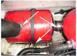
4.1 (Above) Start by removing the waterbox. This will ease removal of the exhaust pipe later. Remove the restraining strap and the two hoses connected at either ends. Loosen the clamps with a screwdriver. Twist the waterbox side-to-side, and pull up from the rear to remove it from the hull.
