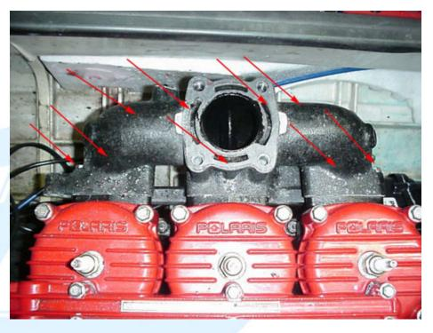
4.8 (Above) Each cylinder has 3 bolts; two at the top and one at the bottom. Remove the bottom and outermost two bolts (short) with a 12mm socket, and loosen the four innermost bolts (long) using a 13mm socket.
