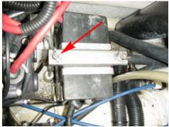
1.1 (Above) Loosen the front retaining wing nut, swing the retainer plate back and remove the plastic protective cover.
