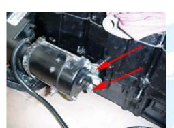
6.6 (Below) Next remove the 4 bolts holding the flywheel case to the crankcase, using a 13mm socket. Then, loosen the 3 Allen head bolts to free the flywheel case from the engine. Remove the starter bendix, and punch out the crank seal, replacing it with a new one.
