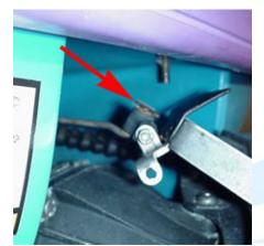
2.4 (Above) Remove the reverse clip by bending the top tab and pushing the clip towards the bend to clear the pivot rod. It's easiest to use needle nose pliers to gently pry the top of the clip up while pushing to release it. After releasing the clip, slide the pivot rod out of the bushing from the bottom.
