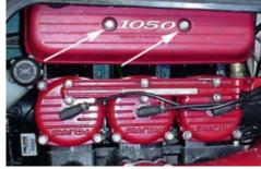
3.2 (Above) Remove the flame arrestor cover bolts with a 13mm socket.
