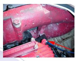
4.5 (Below) Remove the top Exhaust bolts with a 19mm socket and wrench. Remove the pipe from the hull.
