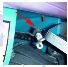
2.4 (Below) On the inside of the hull, at the rear, the cooling water intake and bilge hoses need to be removed. Loosen the hose clamps with a screwdriver, then work the hoses off the nipples.
