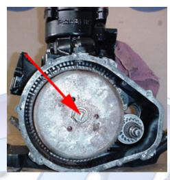
6.9 (Above) Use a universal flywheel puller to remove the flywheel from the crankshaft.
