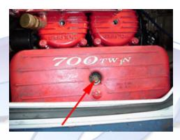
3.2 (Below) Remove the four 10mm bolts securing the velocity stacks and carbs to the intake manifold and remove the stacks.
