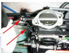
Loosen the gas tank cap to relieve pressure. Be sure the fuel switch is turned to the "OFF" position, and be aware of any fuel that may spill from the hoses. Make sure the hull is clear of any gasoline fumes before continuing work, especially with power tools. Remove the fuel in, fuel return, pulse and oil injection lines from the carbs.
