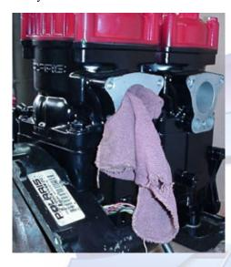
6.7 (Below) Remove the seven 10mm bolts securing the flywheel cover and remove it.
