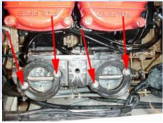
3.3 (Below) Remove the throttle, oil pump and choke cables from the carburetor Pivot the shafts for easy assembly. removal of the cable end-barrels.
