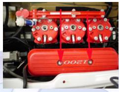
2.6 (Below) Remove the six 10mm bolts securing the throttle bodies to the intake manifold. Disconnect the quick connect to the air flow sensor. Remove the airbox base and bolts from the hull.
