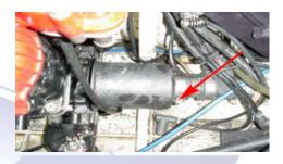
4.5 (Below) Remove the four 19mm nuts from the engine mounts.
