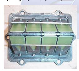
5.3 (Below) Look at each petal-to-cage surface and check for gap. If a gap of more than 0.015" is present, replace the petals.
