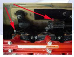
4.3 (Below) Loosen but do not remove the two 13mm bolts holding the PTO shroud in place. Remove the PTO shroud from the hull.
