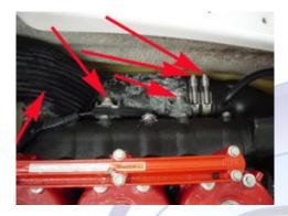
2.4 (Below) Remove the nine 13mm bolts securing the exhaust manifold to the engine. Disconnect the quick connect to the manifold. Remove the exhaust manifold from the hull.
