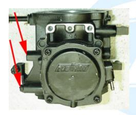
1.2 (Below) Remove the four screws securing the regulator cover and remove it.
