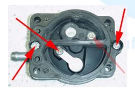
1.10 (Below) Remove the pump diaphragm and o-ring.
