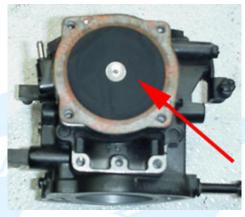
1.4 (Below) Remove the screw retaining the regulator arm assembly. Remove the arm, spring and pull the needle out.
