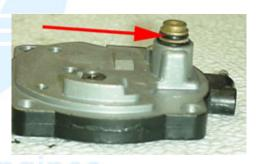
1.7 (Below) Remove the o-ring from the circuit chamber. Remove the two screws securing the high-speed circuit to the chamber and remove the plate. Remove the gaskets and film-valve.
