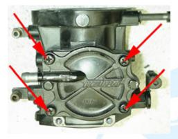
1.9 (Below) Remove the two screws and nuts securing the check valves in place and remove them. Use a Tamper Proof Torx bit to remove the two outer screws and split the pump body. Remove the pump
