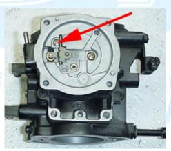
1.5 (Below) Remove the center screw holding the regulator chamber to the carb and remove it. Remove the fuel filter.
